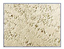
Limestone can be left with rougher surfaces, or dressed to a smoother finish using hand and power tools, and it is even able to be turned and made into columns.
